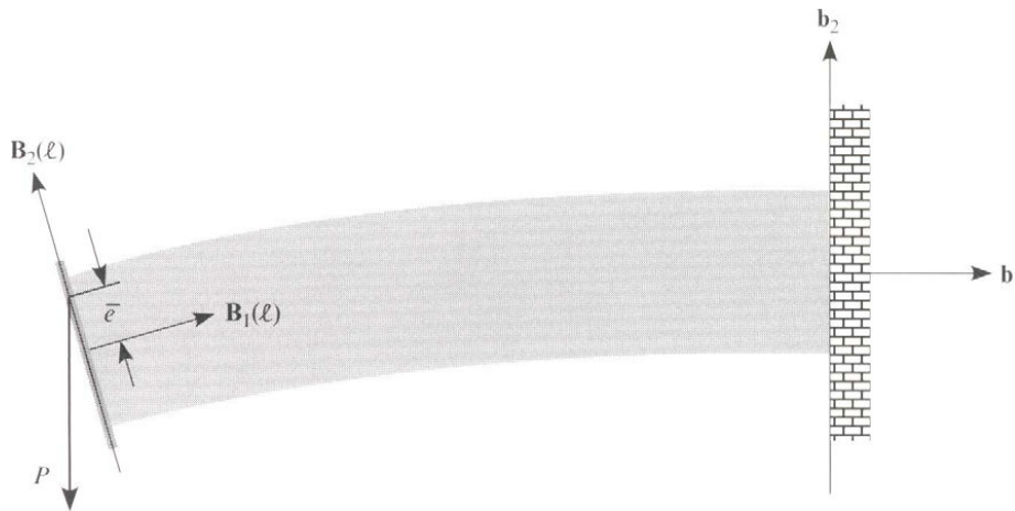
FIGURE 9.4 Schematic of end-loaded cantilever
